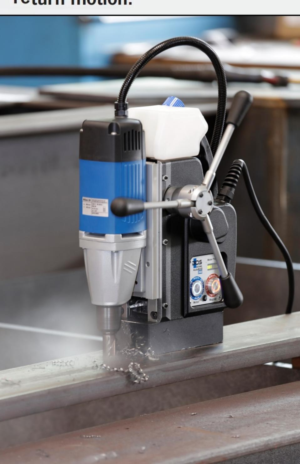
Feed is activated when the handles are pressed. The drilling procedure is monitored by the control and the load is indicated by the LED bar. At the end of the drilling procedure, the motor automatically moves back into the zero position.
